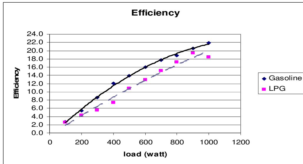
Figure 5.22: Comparison of engine efficiency of gasoline and LPG fuel system
